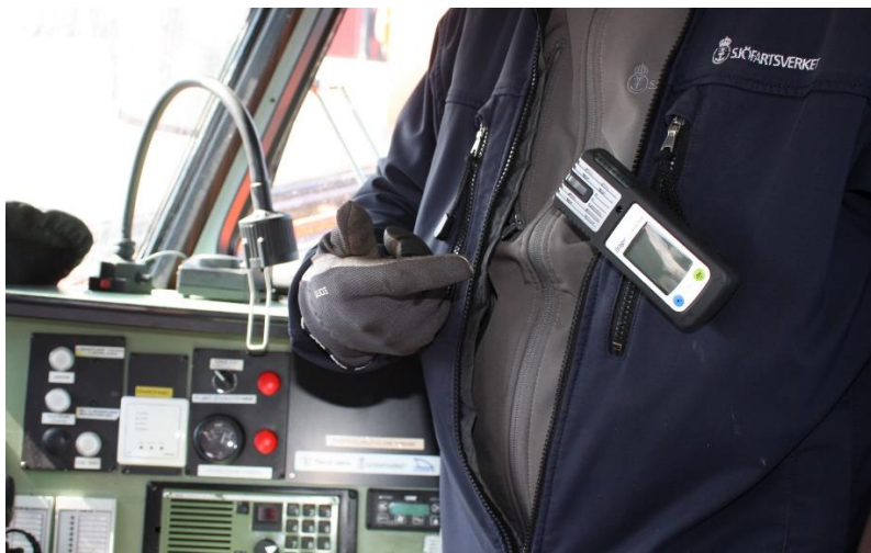
Figure 6. Ex classed portable gas detector used on the Swedish Maritime Administration's Pilot Boat 120 SE
